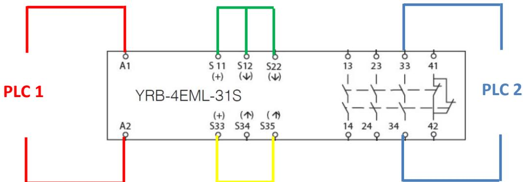
Fig 15 – Wiring with 2 PLCs
