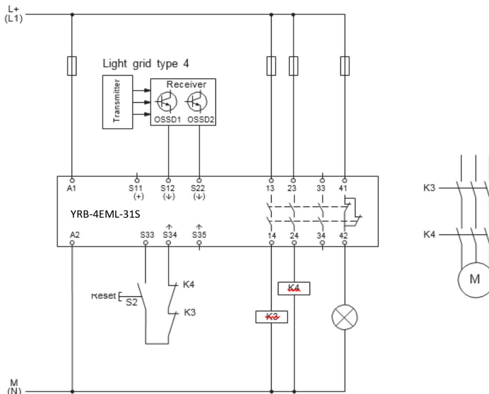
Figure 13 Two-channel light curtain monitoring with manual reset YRB-4EML-31S
