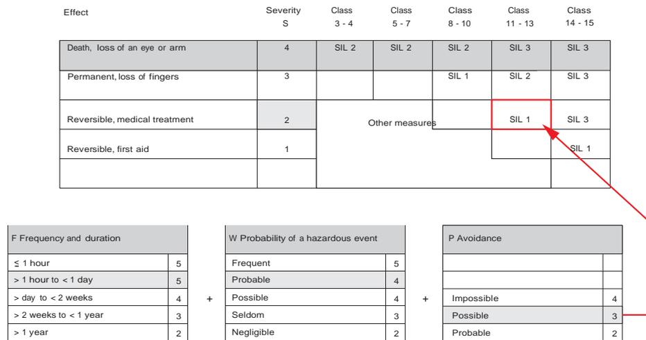
Figure 5 Example of specifying the SIL (according to EN 62061)
