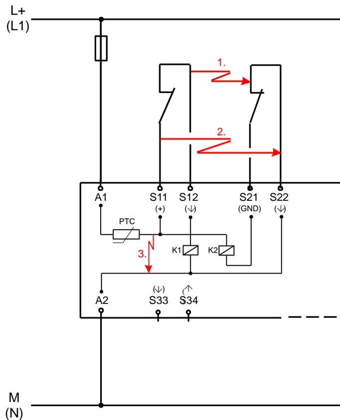
Figure 6 Cross-circuit detection
