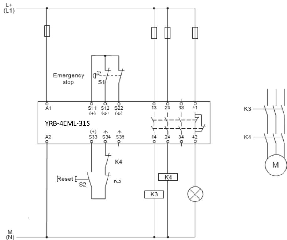
Figure 12 Two-channel emergency stop monitoring with manual reset YRB-4EML-31S
