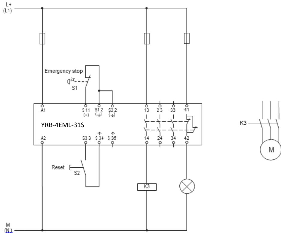
Figure 11 Single-channel emergency stop monitoring with manual reset
