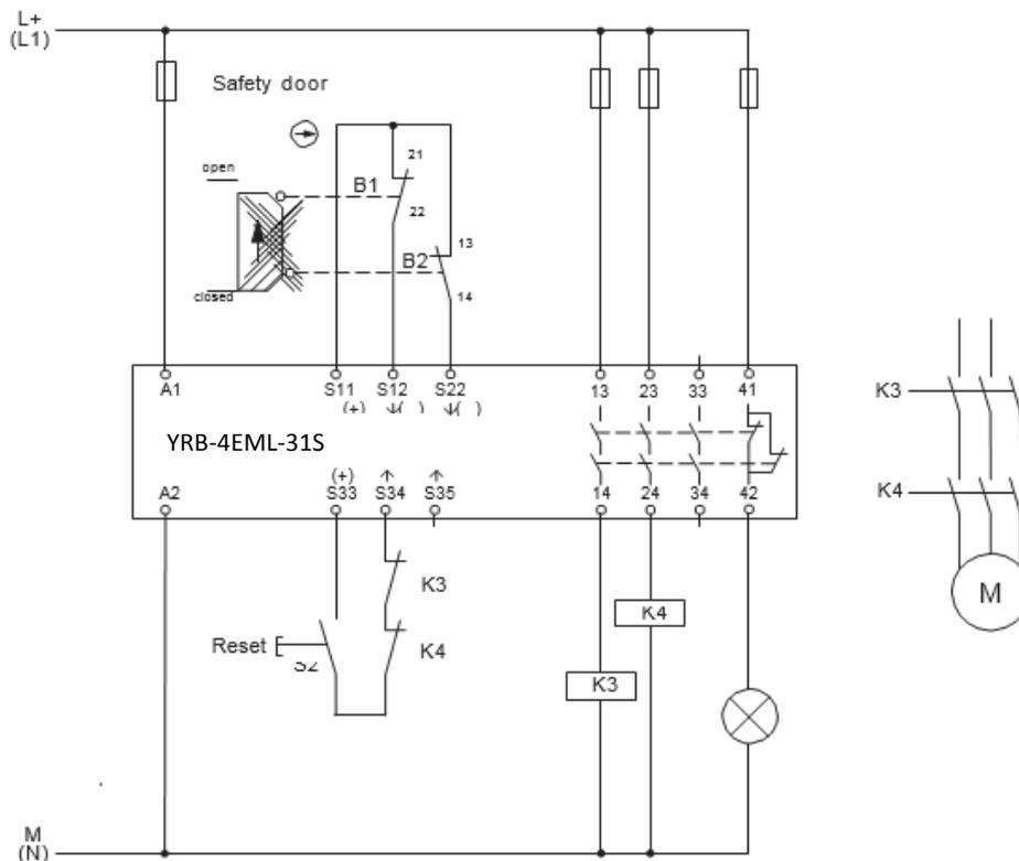
Figure 14 Two-channel safety door monitoring with manual reset YRB-4EML-31S
